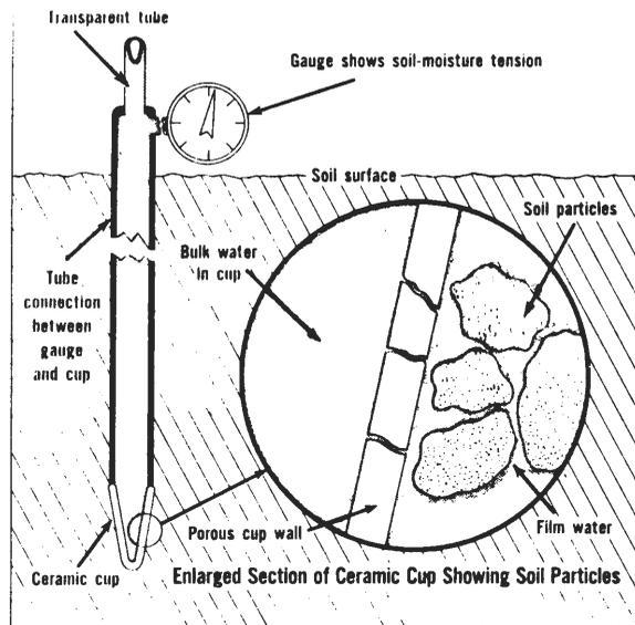
Figure 1. Cross section of a tensiometer
