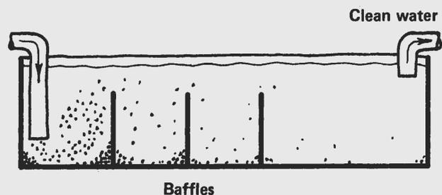
**SETTLING BASIN**—the longer and deeper the better, but build so sediment can be cleaned out.
