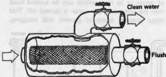
**SCREEN FILTER**—available commercially in singles, multiples, and automated for reverse flushing.
