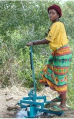
A Malawi woman uses a treadle pump for small-scale irrigation.
