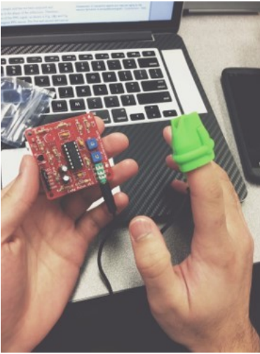
Viable prototype of the Cardio One, VB Cardio's blood pressure monitor that can be worn on a finger
