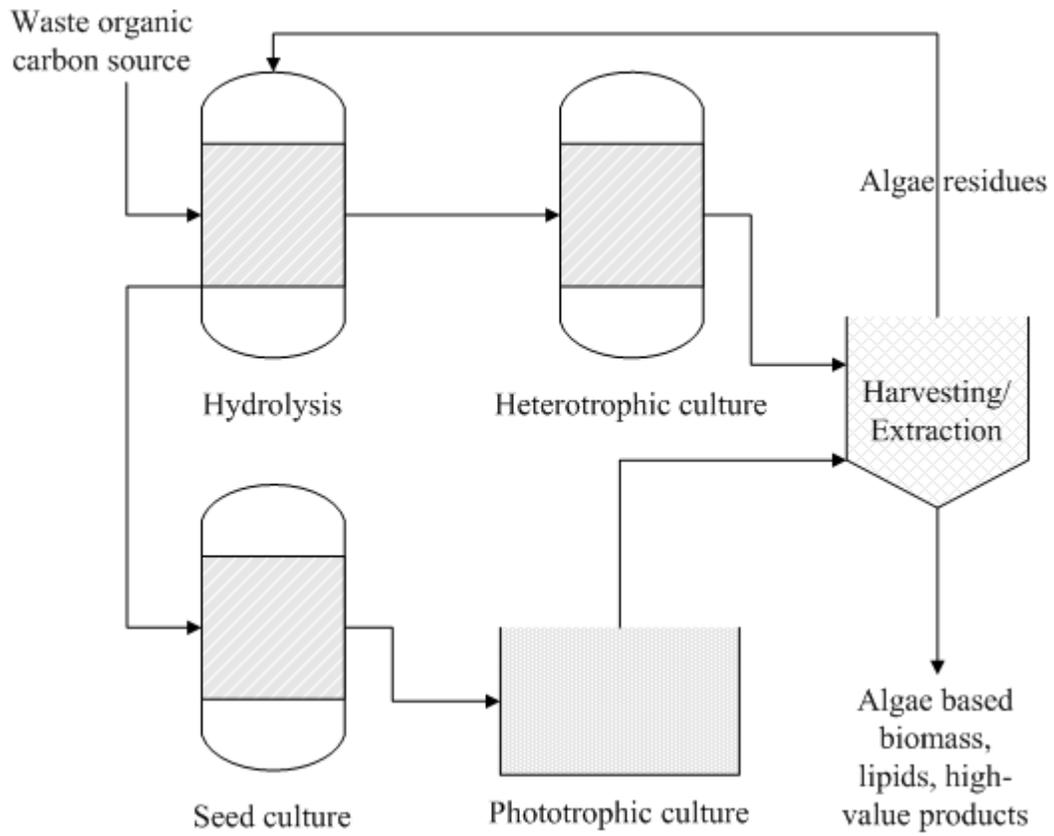
Fig. 1.2. Overview for an integrated system of the two-stage heterotrophic and phototrophic culture of microalgae
