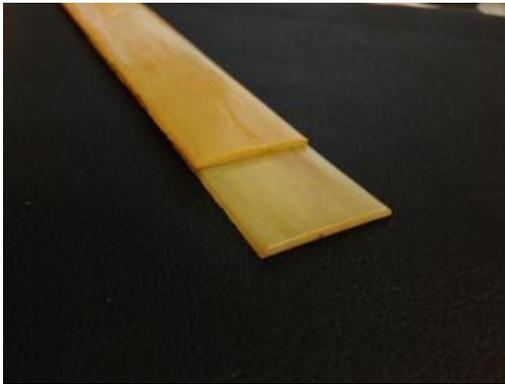
Fig. 5: Pultruded glass fiber/bio-based polymer composites
