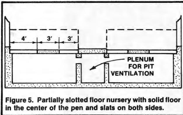
Figure 5. Partially slotted floor nursery with solid floor in the center of the pen and slats on both sides.
