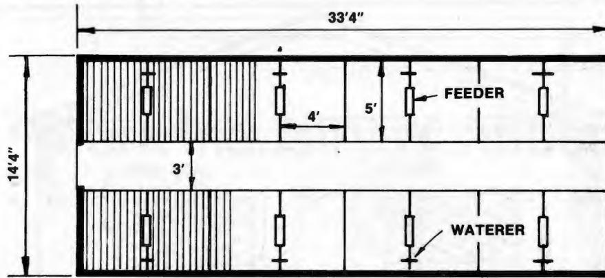
Figure 6. Slotted floor nursery for individual litters. Flooring material with 50-60% open area is desirable.
