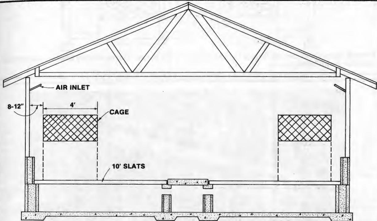
Figure 7. Cages for weaned pigs before transferring to the slotted floor below.
