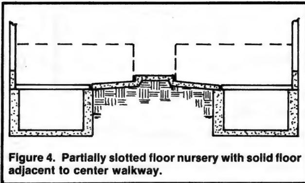
Figure 4. Partially slotted floor nursery with solid floor adjacent to center walkway.
