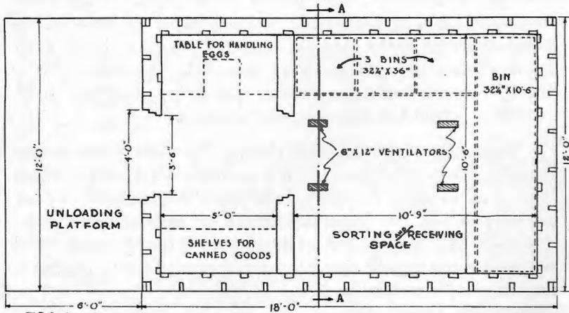
FIG.1 FLOOR PLAN
