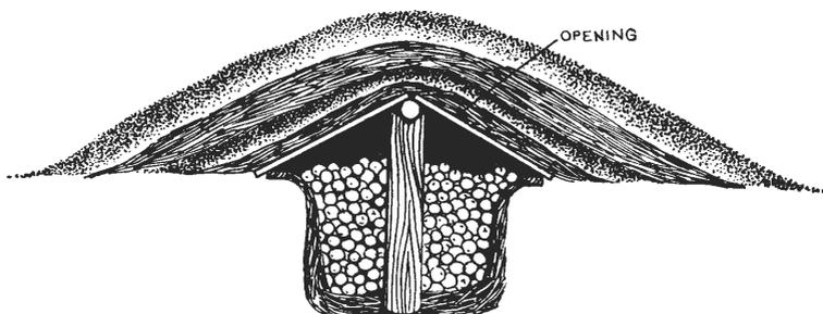
Fig. 5. Shallow pit storage with roof support. Same as Figure 4 with the addition of a roof support. The roof support keeps covering from caving in as products are removed.
