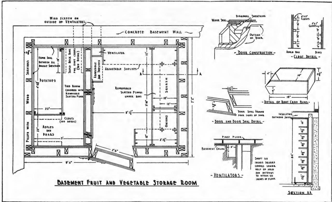
Fig. 2. Basement fruit and vegetable storage with a humid and a dry room. Bins for carrots, beets, parsnips and similar root crops are in the form of drawers, one above another. Shelf cleats for apple boxes are built in. Shelf arrangement in dry room is the same as for the above ground storage, shown in Figure 1, except that a section of shelves for jam is added.
