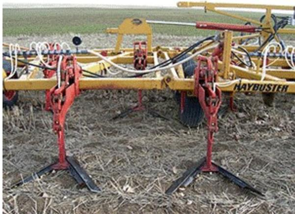
An undercutter with V-shaped blades is used for primary spring tillage with fertilizer injection added during the fallow year.
