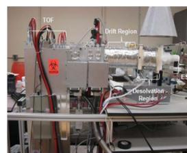
Figure 4: Instrument image of AP-IM-TOFMS
