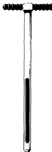
Figure 2. An open-face sampling tube, the tool most commonly used for most situations. The tip is slightly enlarged on the outside and slightly tapered inward on the inside for efficient sample extraction.
