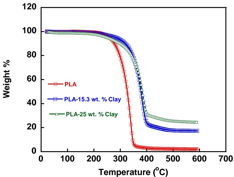
**Figure 4:** TGA curves of PLA and PLA/clay nanocomposites with different clay loadings.
