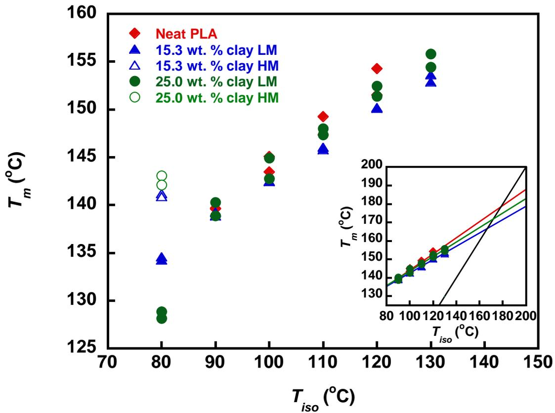
**Figure 7:** Relationship between  $T_m$  and  $T_{iso}$  for PLA and PLA/clay nanocomposites. The letters LM and HM represent the peak temperatures of the low and high temperature endotherms, respectively. The result of Hoffman Weeks method for the determination of  $T_m^0$  is shown in the inset.
