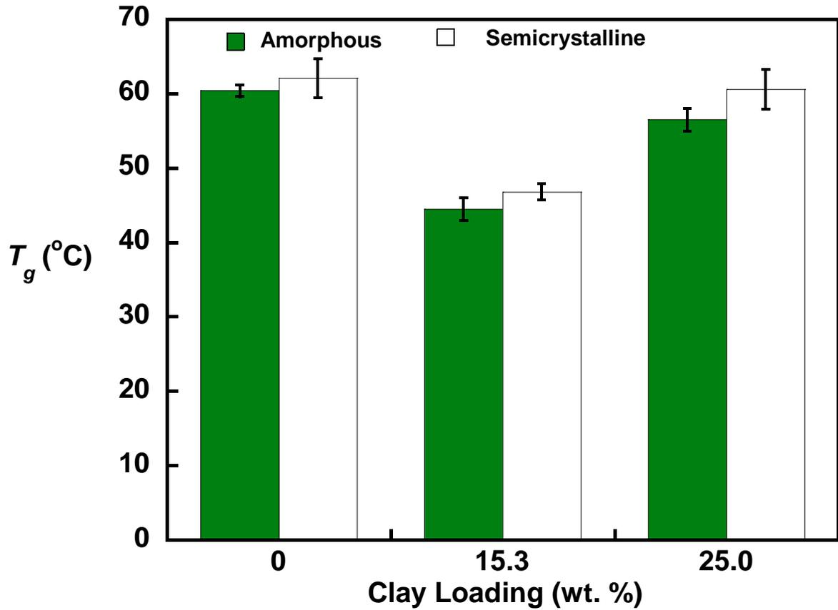
**Figure 10:** Effect of clay loading on glass transition temperature ( $T_g$ ) of PLA and PLA/clay nanocomposites. The values for amorphous  $T_g$ s were obtained based on three measurements for each sample. The values of semicrystalline  $T_g$ s were based on four measurements at 100  $^{\circ}\text{C}$ , following complete crystallization. The error bars represent standard deviations of the measurements.
