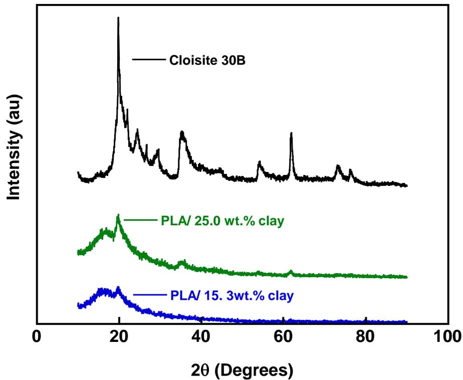
**Figure 3:** XRD spectra of neat PLA compared with PLA/clay nanocomposites
