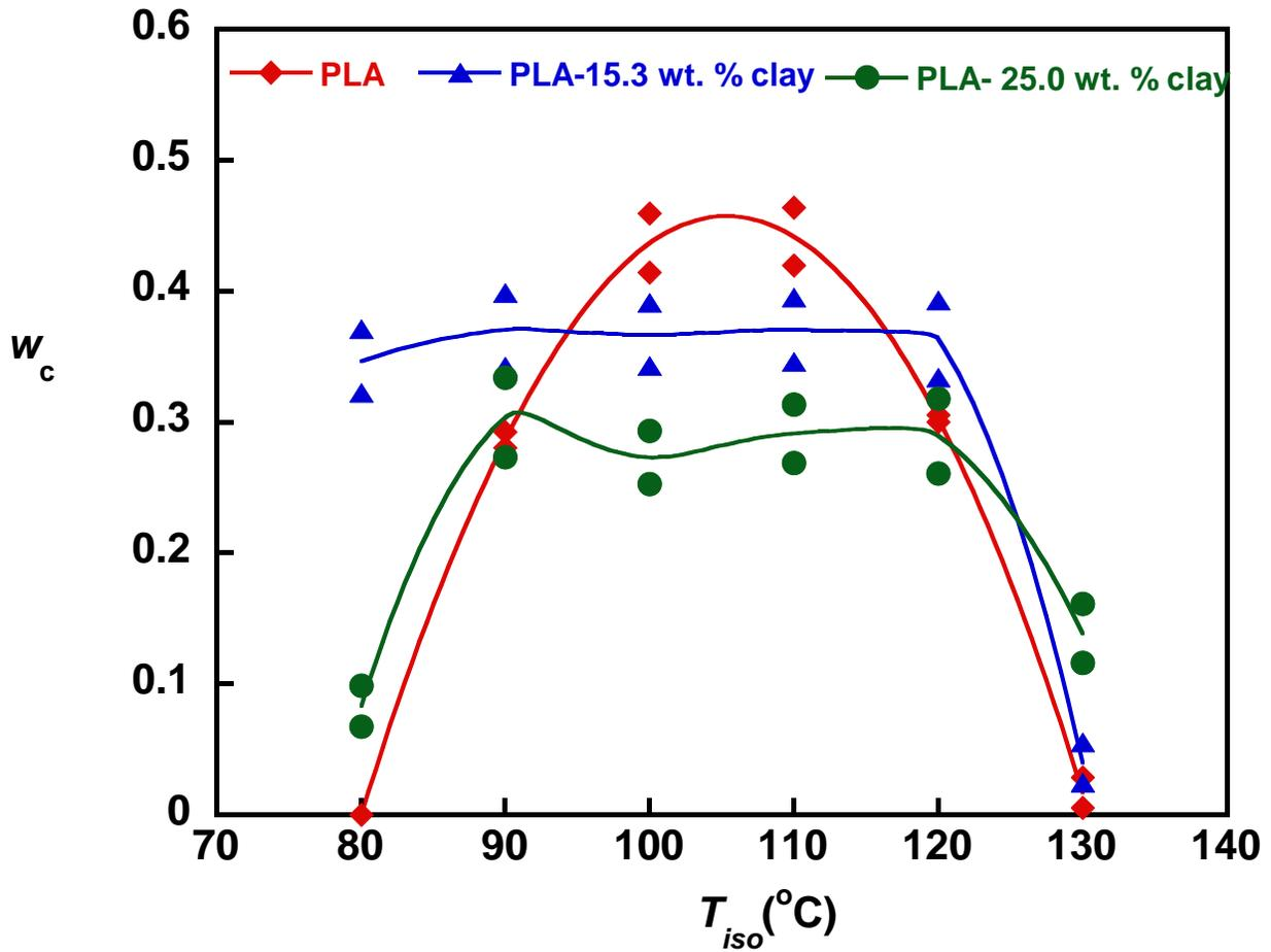
**Figure 8:** A comparison of crystallinity for PLA and PLA/clay nanocomposites obtained on heating at 500 °C/min following isothermal melt crystallization at various values of  $T_{iso}$  for 60 min. Lines are drawn as a visual guide. Two specimens were characterized at each  $T_{iso}$  for all three sample types (i.e., 0 wt. % clay, 15.3 wt. % clay, and 25.0 wt.% clay).
