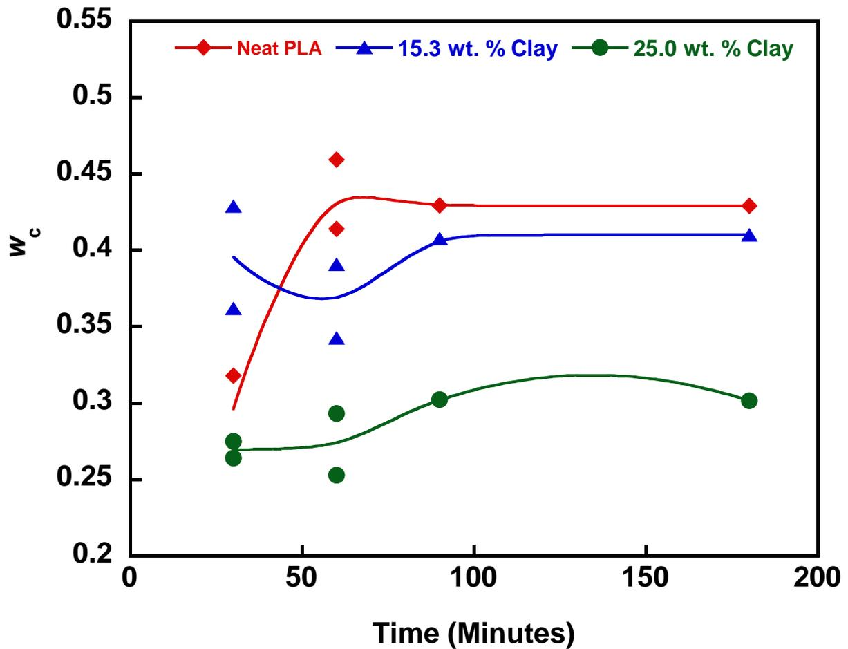
**Figure 9:** A comparison of crystallinity for PLA and PLA/clay nanocomposites obtained on heating at 500 °C/min following isothermal melt crystallization at  $T_{iso} = 100$  °C for various periods from 30 to 180 min. Two specimens were characterized at isothermal periods of 30 min for all three sample types. For isothermal periods longer than 60 min, no change in  $w_c$  was observed and only one measurement was performed.
