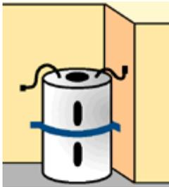
Most water heaters have sections of flexible tubing to make replacement easier. Flexible tubing also helps during an earthquake when movement occurs. Some older installations may not have flexible lines. Consider installing flexible lines if you replace the water heater. Add strapping material to help hold the water heater upright. This reduces the chance of a hot water heater falling over.
