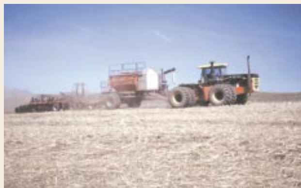
Melvilles’ Yielder no-till drill seeding peas into grazed barley stubble, with inset of N-P opener (top), and their Concord no-till drill seeding spring wheat into spring barley stubble.
