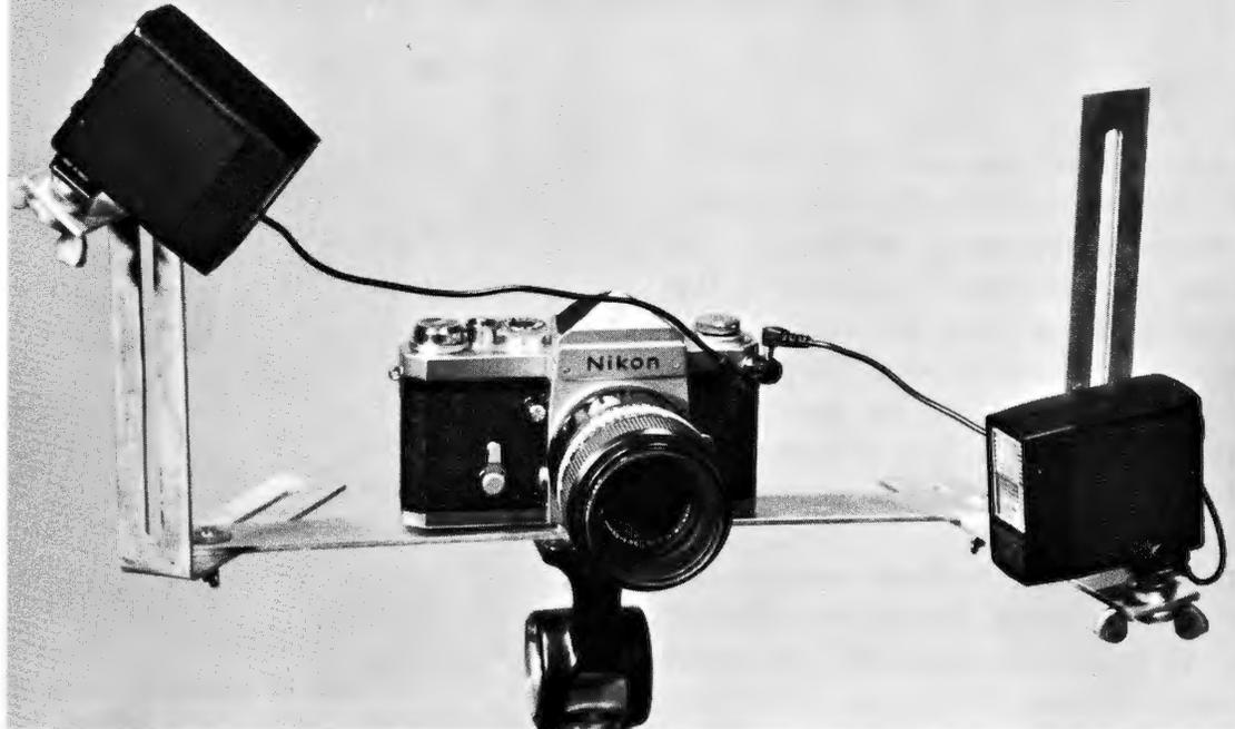
Figure 2. Camera with flash holders and electronic flashes ready for use.
