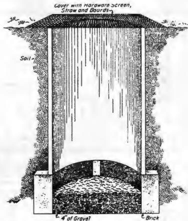
Fig. 8. Tile storage pit . A convenient and fairly permanent storage unit can be made by setting a large tile into the ground.
