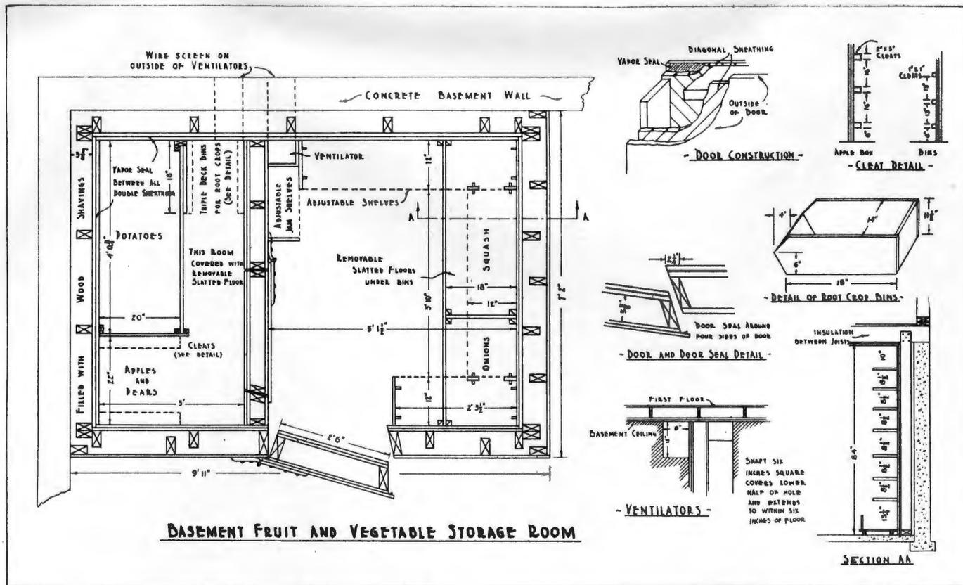
Fig. 10. Basement fruit and vegetable storage with a humid and a dry room. Bins for carrots, beets, parsnips and similar root crops are in the form of drawers, one above another. Shelf cleats for apple boxes are built in. Shelf arrangement in dry room is the same as for the aboveground storage shown in Figure 9, except that a section of shelves for jam is added.
