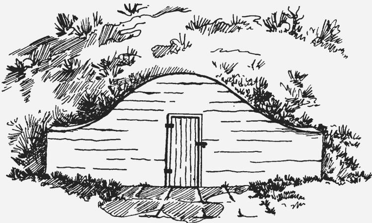
Fig. 6. Side hill storage. Common in areas where the land is rolling. The inside arrangement suggested in Figure 9 may be used.
