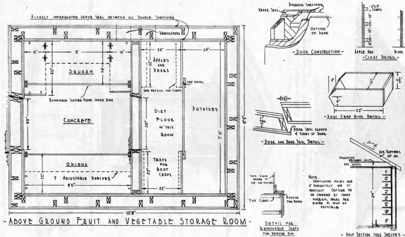
Fig. 9. Aboveground fruit and vegetable storage, separate from the house. Note moist room for high humidity crops and dry room for low humidity crops. Shelves in dry room for canned goods are removable; those in one section are adjustable. Bin partitions are removable to aid in keeping the storage clean.
