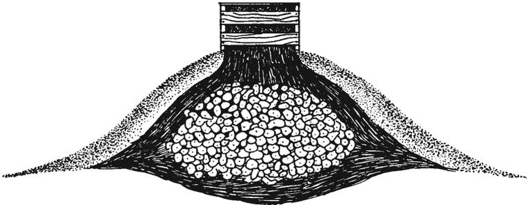
Fig. 2. Small pit above ground level, with apple box ventilator in place. Ventilator is put on when pit is made and vegetables are put in; it allows field heat of vegetables to escape and cold air to enter.
