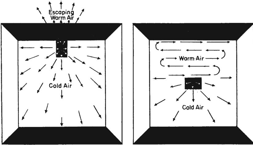
Fig. 1. Drawings showing right and wrong location for ventilator. When ventilator is placed near ceiling all warm air can escape.
